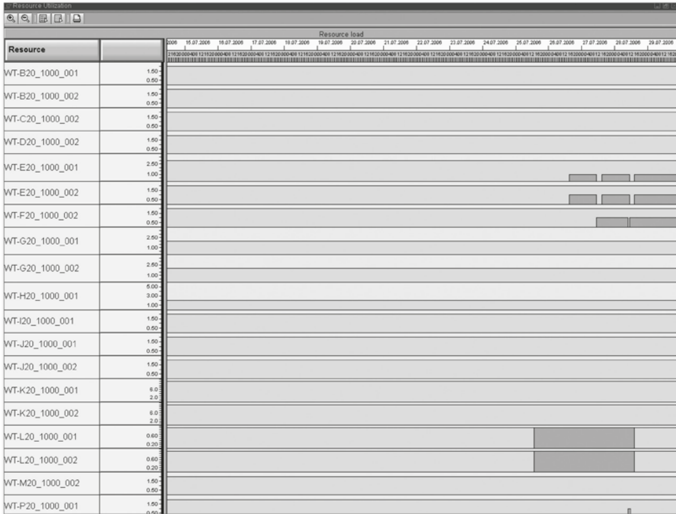
Figure 7.10 APO Transaction "Detailed Scheduling Planning Board," Transaction Code /SAPAPO/CDPS0, "Resource Utilization" Chart Overloads No Longer Occur in the Optimization Period
