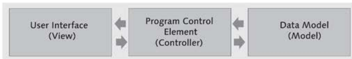
Figure 1.1 Simplified Representation of the MVC Architecture Pattern
