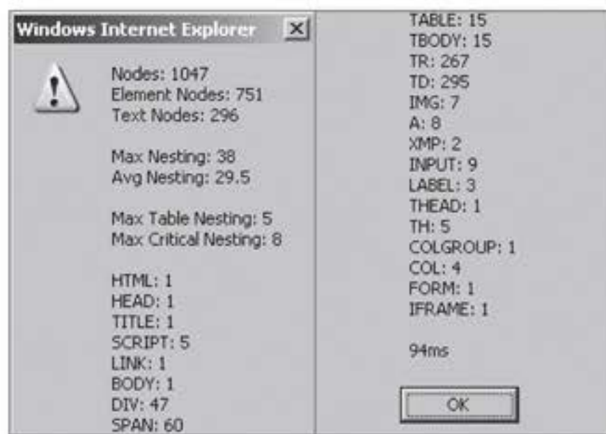
Figure 8.6 DOM Analysis for a Web Dynpro Application
