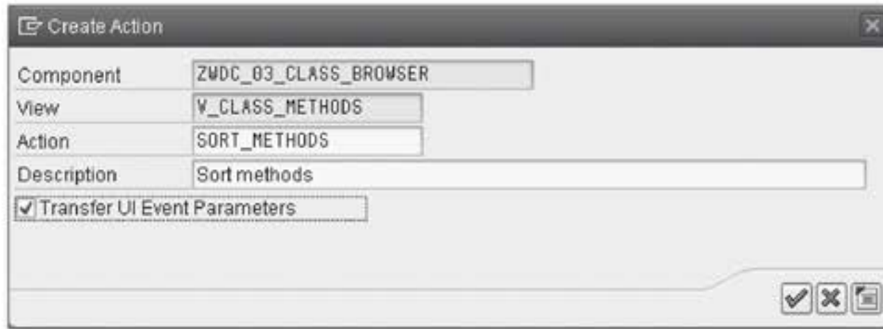
Figure 3.65 Creating the SORT_METHODS Action for the onSort Event of the Table UI Element
